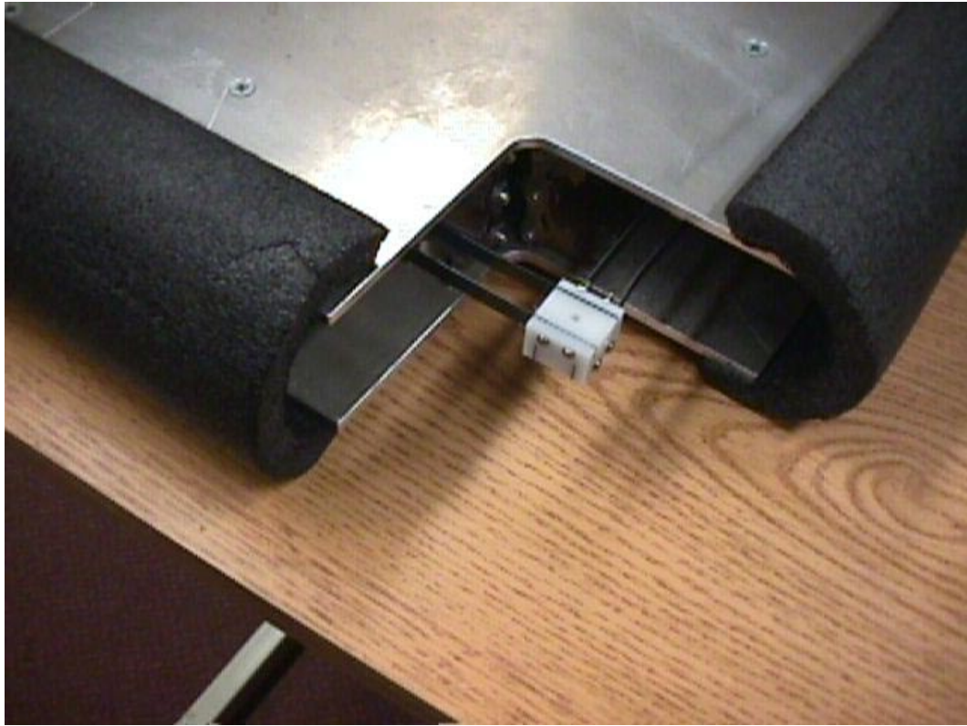
Fig. 4.3. Prototype haptic display device: the Moose. Two linear voice-coil motors are coupled to the white puck in the center of the Moose’s workspace by two perpendicularly-oriented double flexures. The puck’s position is tracked by two linear encoders and the whole is interfaced to the host computer via a digital I/O card.
