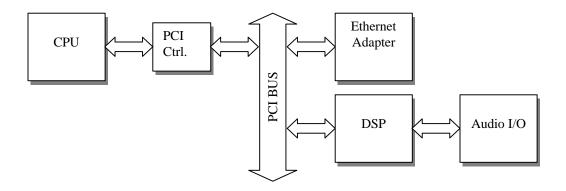
Topology of an Embedded System for Audio Applications
