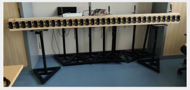
Prototype of an FPGA-based WFS system (programmed in Faust) using cheap (\$6, well \$3 a year ago lol) Adafruit i2s amplifiers (MAX98357A):
