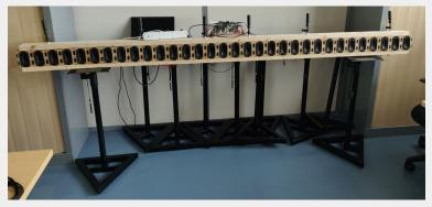
Prototype of a SyFaLa-based WFS system (programmed in Faust) using cheap (\$6, well \$3 a year ago lol) Adafruit i2s amplifiers (MAX98357A):
