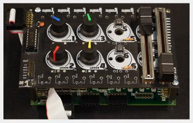
Sister board provided as part of SyFaLa. It is based on a TI sensor ADC and it can host various controllers: push buttons, rotary and linear potentiometers, etc.
