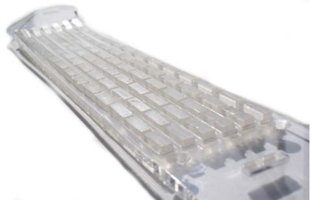
Figure 7. BLADEAXE neck based on silicon buttons. Buttons were 1/8” high.
