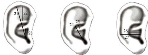
Figure 2: Examples of measurements that determine pinna coefficients in a hypothetical parametric HRTF
