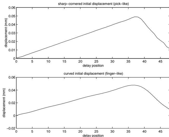
**Fig. 1.** (Top) Sharp-cornered initial displacement for pick-like simulation. (Bottom) Low curvature initial displacement for finger-like simulation.
