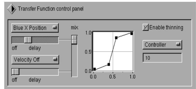
As before, a mix of velocity and position information is fed to the transfer function which is used to generate a continuous MIDI information stream (pitch bend, pressure or continuous controllers).
