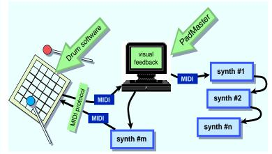
ON or OFF the communication program, set the MIDI channel used by the rest of the protocol, dump and load the internal calibration tables, set the trigger and release heights for both batons, request raw A/D measurements (useful for testing), etc.
