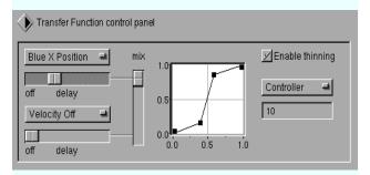
As before, a mix of velocity and position information is fed to the transfer function which is used to generate a continuous MIDI information stream (pitch bend, pressure or continuous controllers).
