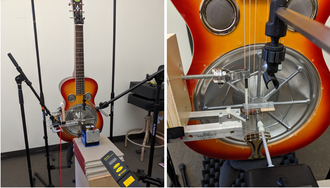
Figure 1. Measurement Setup showing the LDV, force hammer, and shaker. Note, the shaker's force sensor is not shown.
