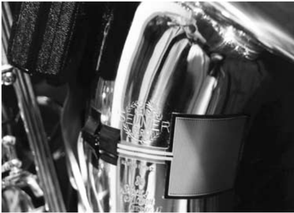
Figure 6. Bell of the Metasaxophone showing the microprocessor casing, the front bell trigger sensor, and the Selmer Insignia.
