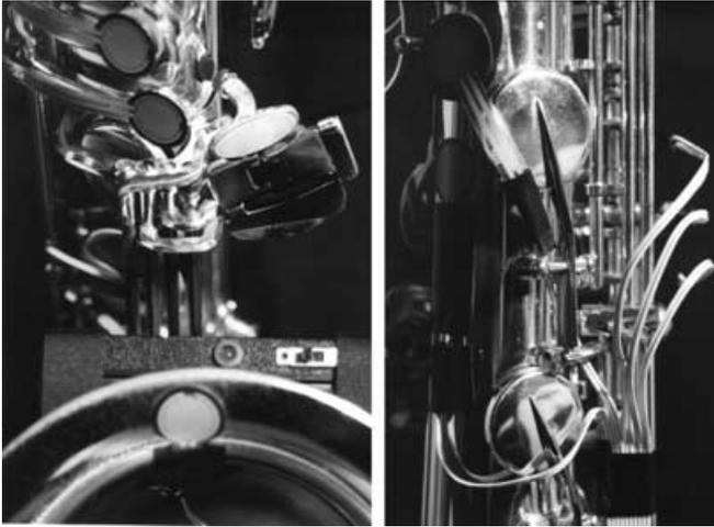
Fig. 6. The metasaxophone: front and back views.
