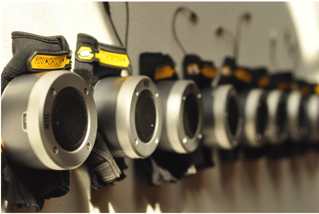
Figure 4: Selected Prototype Design: Speaker gloves
