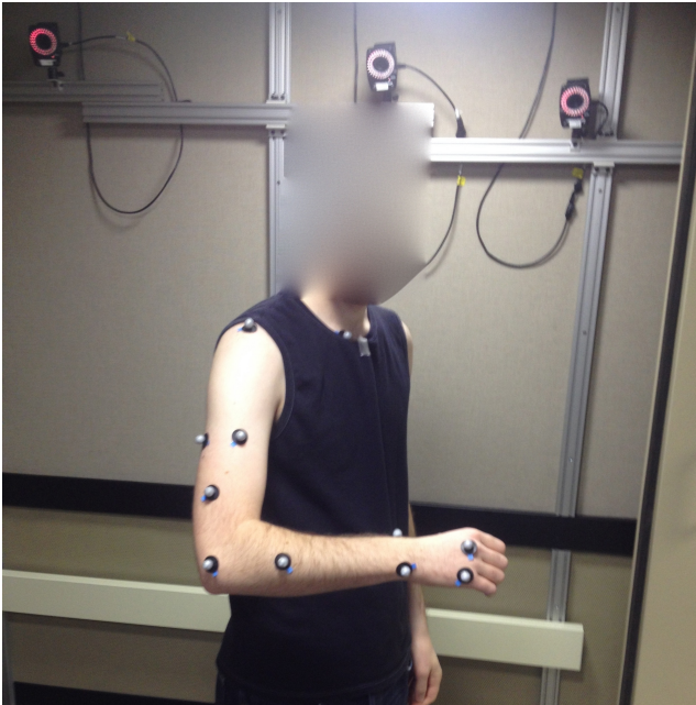
Figure 2: A participant with markers and motion capture cameras
