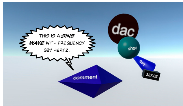
Figure 3. Audio comments in VRAPL allow users to leave verbal descriptions to be played back later. This comment will play back a recording that says, 'this is a sine wave with frequency 337 Hz'.
