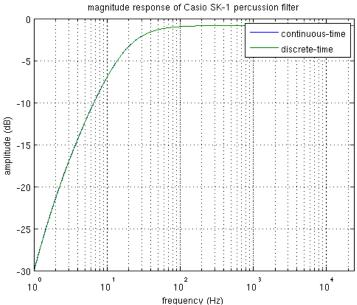
The filter is clearly a high-pass filter. By inspection, the cutoff frequency is around  $200\,Hz$  and the filter has a low-frequency roll-off of  $12\,dB/octave$  or  $40\,dB/decade$ .
