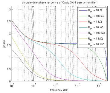
It will be useful to find the value of resistor  $R_{44}$  that is required to produce a filter with a desired cutoff frequency. The equation for the cutoff frequency in Hertz  $(f_c)$  is revisited, solving for  $R_{44}$  in terms of the desired cutoff frequency and component values:
