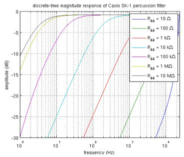
By inspection, a ten-fold increase in the resistance of  $R_{44}$  generally corresponds to a ten-fold decrease of the cutoff frequency of the filter, and a ten-fold decrease in the resistance of  $R_{44}$  generally corresponds to a ten-fold increase of the cutoff frequency. This behavior is somewhat different around DC and the Nyquist frequency.
