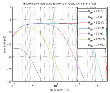
By inspection, a ten-fold increase in the resistance of  $R_{30}$  generally corresponds to a ten-fold decrease of the bandwidth of the filter, and a ten-fold decrease in the resistance of  $R_{30}$  generally corresponds to a ten-fold increase of the bandwidth. This behavior is somewhat different around DC and the Nyquist frequency.
