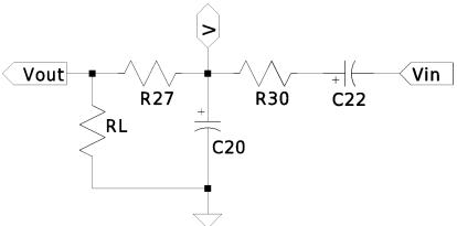
The only difference from the Bass Filter is that the components are named differently, and one has a different value. Component values as given in the Realistic Concertmate-500 service manual:
