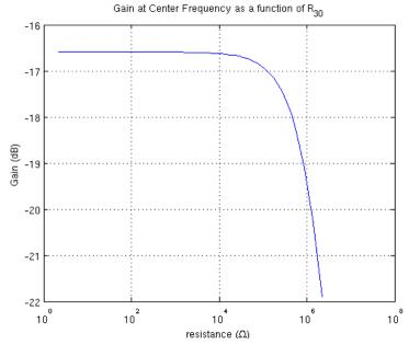
The gain is not affected very much, unless  $R_{30}$  gets above  $100k\Omega$  (corresponding to a very low Q). This can be seen on the graph of the magnitude response as well.
