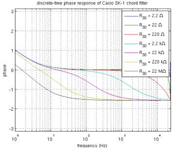
It will be useful to find the value of resistor  $R_{30}$  that is required to produce a filter with a desired Q. The equation for Q is revisited, solving for  $R_{30}$  in terms of the desired Q and component values:
