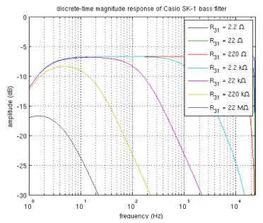
By inspection, a ten-fold increase in the resistance of  $R_{31}$  generally corresponds to a ten-fold decrease of the bandwidth of the filter, and a ten-fold decrease in the resistance of  $R_{31}$  generally corresponds to a ten-fold increase of the bandwidth. This behavior is somewhat different around DC and the Nyquist frequency.
