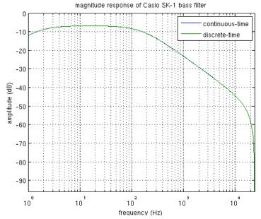
The Bass Filter is clearly a band-pass filter. By inspection, the cutoff frequency is around  $20\,Hz$  and the filter has a high-frequency roll-off of  $6\,dB/octave$  or  $20\,dB/decade$  (and, presumably, an identical low-frequency roll-off).
