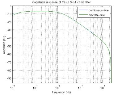
The Chord Filter is clearly a band-pass filter. By inspection, the cutoff frequency is around  $20\,Hz$  and the filter has a high-frequency roll-off of  $6\,dB/octave$  or  $20\,dB/decade$  (and, presumably, an identical low-frequency roll-off).
