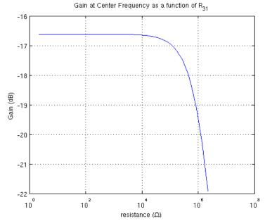
The gain is not affected very much, unless  $R_{31}$  gets above  $100k\Omega$  (corresponding to a very low Q). This can be seen on the graph of the magnitude response as well.
