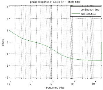
For both the magnitude and phase responses, there is no visible difference between the plots for the continuous-time and discrete-time filters, so the bilinear transform is assumed to be an approximation of high enough order to well-describe this system. Presumably, frequency warping is not an issue for low-order filters.
