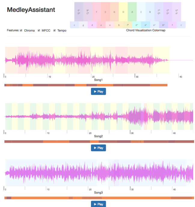
Figure 1. MedleyAssistant Interface. For each song, we visualize chords (as colored blocks on the waveform) and tempo (as a color density bar below the waveform).
