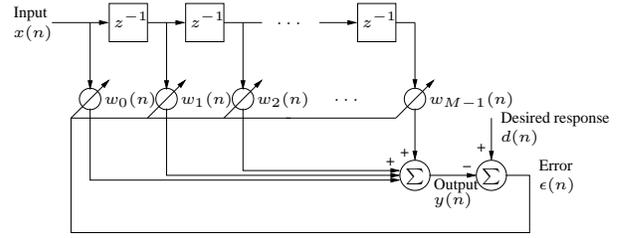
Figure 1: Adaptive linear combiner in the form of single-input adaptive transversal filter (adapted from [7]).
