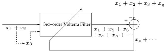
Figure 2: Third-order adaptive Volterra filter with desired response and error signal.  $x_q$  and  $x_c$  indicate the quadratic and cubic difference tone at frequency  $2f_1 - f_2$ , respectively.
