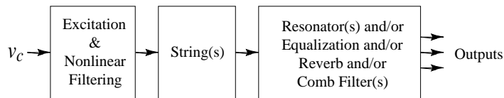
Figure 6: Example block diagram of a complete, commuted-piano synthesis system, including resonators which partially implement the response of the soundboard and enclosure, equalization sections for piano color variations, reverberation, comb-filter(s) for flanging, chorus, and simulated hammer-strike echoes on the string, and multiple outputs for enhanced multi-channel sound.
