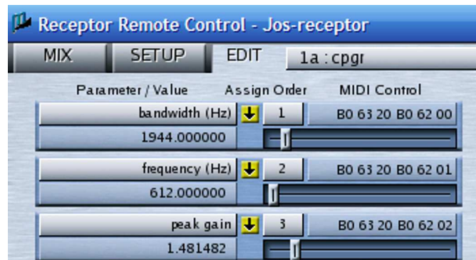
Figure 14: Screenshot of the upper-left corner of the parameter-editing window of the Receptor’s remote-control program showing the constant-peak-gain resonator parameters.
