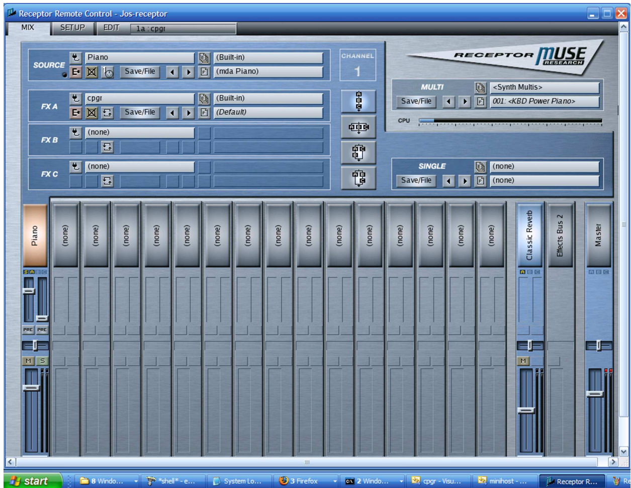
Figure 13: Screenshot of the Receptor Remote Control program, showing the “Mix” view. The constant-peak-gain resonator (named cpgr ) is instantiated as a plugin processing the “Piano” source signal.
