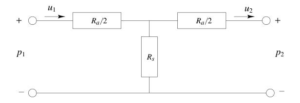
For implementation in a digital waveguide model, the lumped shunt and series impedances must be converted to scattering parameters:
