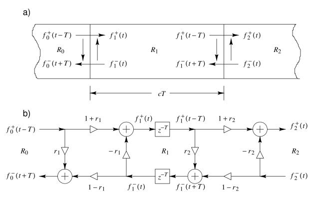
A waveguide section between two partial sections
