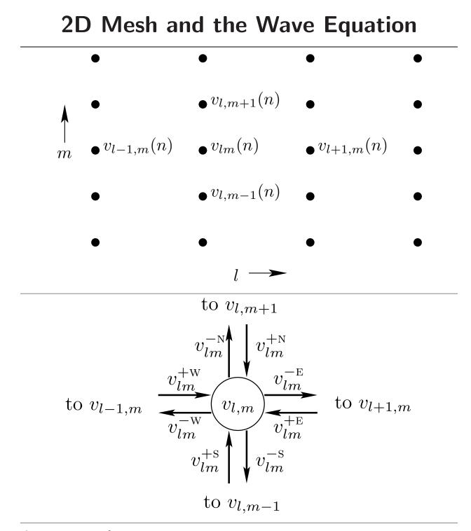
Junction velocity  $v_{lm}$  at time n:
