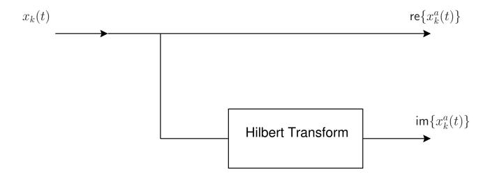
Practical Hilbert transformers may be designed as FIR filters (e.g., firpm in the Matlab Signal Processing Toolbox). (See FIR Hilbert-Transform Design in the lecture on the Window Method for FIR Filter Design)
