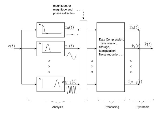
Input signal is decomposed into subbands.
