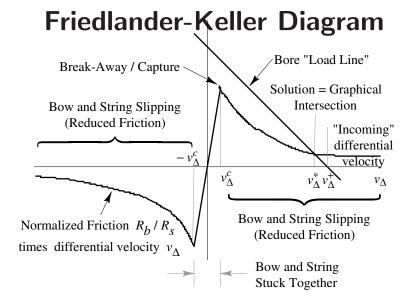
Overlay of normalized bow-string friction curve  $R_b(v_\Delta)/R_s$  with the bore "load line"  $v_\Delta^+ - v_\Delta$ . The "capture" and "break-away" differential incoming velocity is denoted  $v_\Delta^c$ . Note that increasing the bow force increases  $v_\Delta^c$  as well as enlarging the maximum force applied (at the peaks of the curve).
