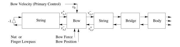
A schematic model for bowed-string instruments.
