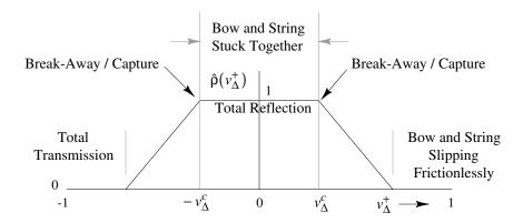
Simple, qualitatively chosen bow table for the digital waveguide violin.
