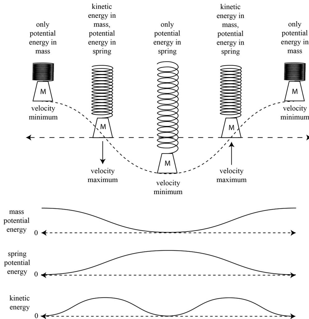
Figure 2: Oscillating mechanical systems interchange kinetic and potential energy - the same principle applies to acoustic systems.
