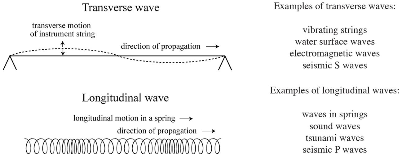
Figure 1: Transverse and longitudinal waves
