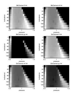
**Figure 4**. Method 1: Timbre difference  $D_{\bar{c}}$  between reference and synthesis sounds. Reference sounds are from a Bb and Eb Clarinet at dynamic levels *ff, mf* and *pp*. The brighter cells correspond to more similarity between reference and synthesis sounds. Note how the distribution of similarity varies with reference sound.
