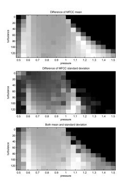
**Figure 5**. Timbre similarity distribution for the B $\flat$  Clarinet *ff* sound measured by, Top: Mean MFCC, Middle: MFCC standard deviation, Bottom: Both.
