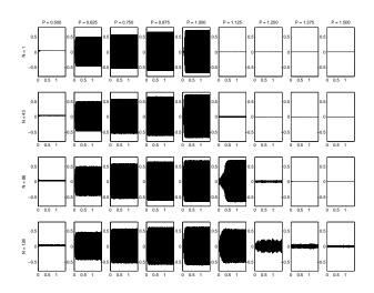
**Figure 1**. Waveforms of clarinet synthesis with increasing blowing pressure from left to right, and noise amplitude increasing from top to bottom. Note that both underblowing and over-blowing do not yield oscillation.
