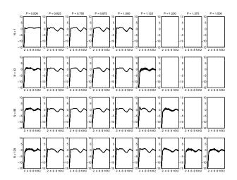
**Figure 2**. MFCC of clarinet synthesis shown in Figure 1. Ten frames are overlaid and the deviation of the MFCC becomes larger as the turbulence grows.
