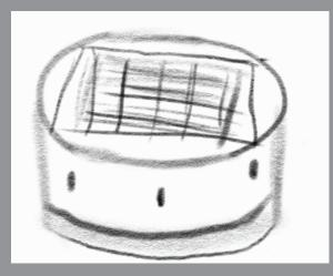
Bluetooth connected microphone assembly adheres to the outside of the car. A solar panel recharges the internal battery, which can be optionally charged by USB. The top portion of the unit screws off the bottom base which is stuck to the top of the vehicle.
