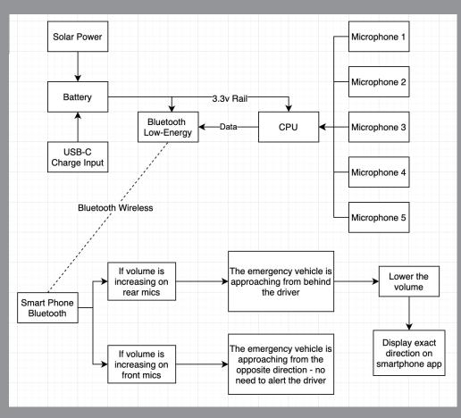
Five microphones detect the intensity and direction of sounds - distinguishing between emergency vehicles behind the driver and in opposite direction on the other side of the road. The driver will only be alerted to vehicles behind them.
