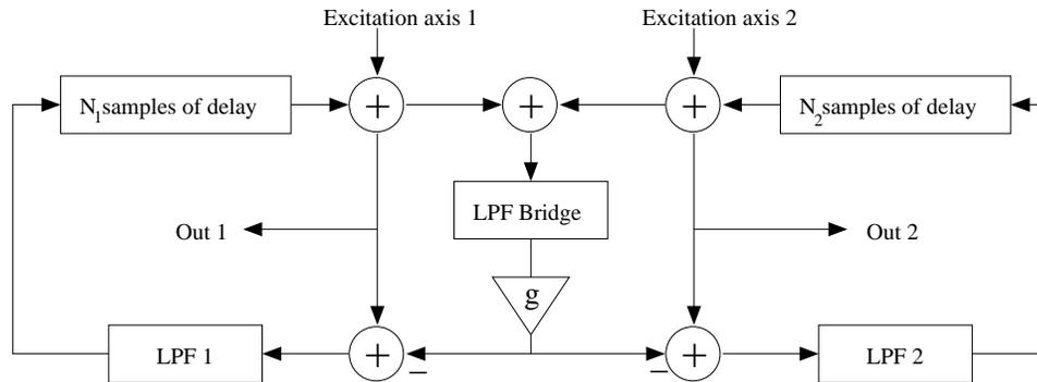
Figure 3: Two axis digital waveguide string model
