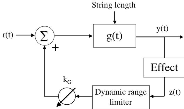
Figure 4: Configuration for sustaining an arbitrary effect.
