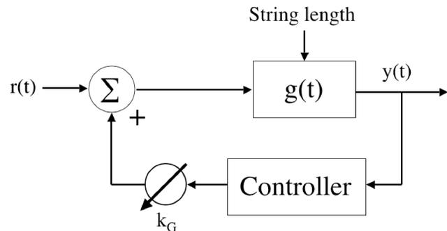
Figure 1: System block diagram for one string.
