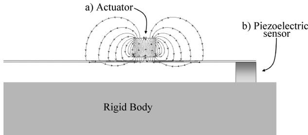
Figure 2: Sensor and actuator placement.
