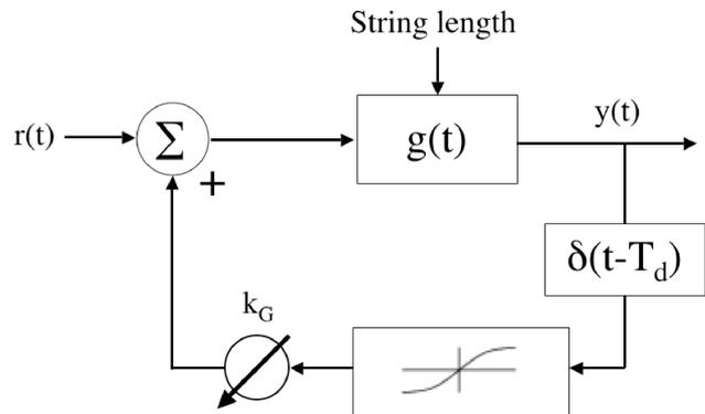
Figure 3: Nonlinear amplifier controller configuration.
