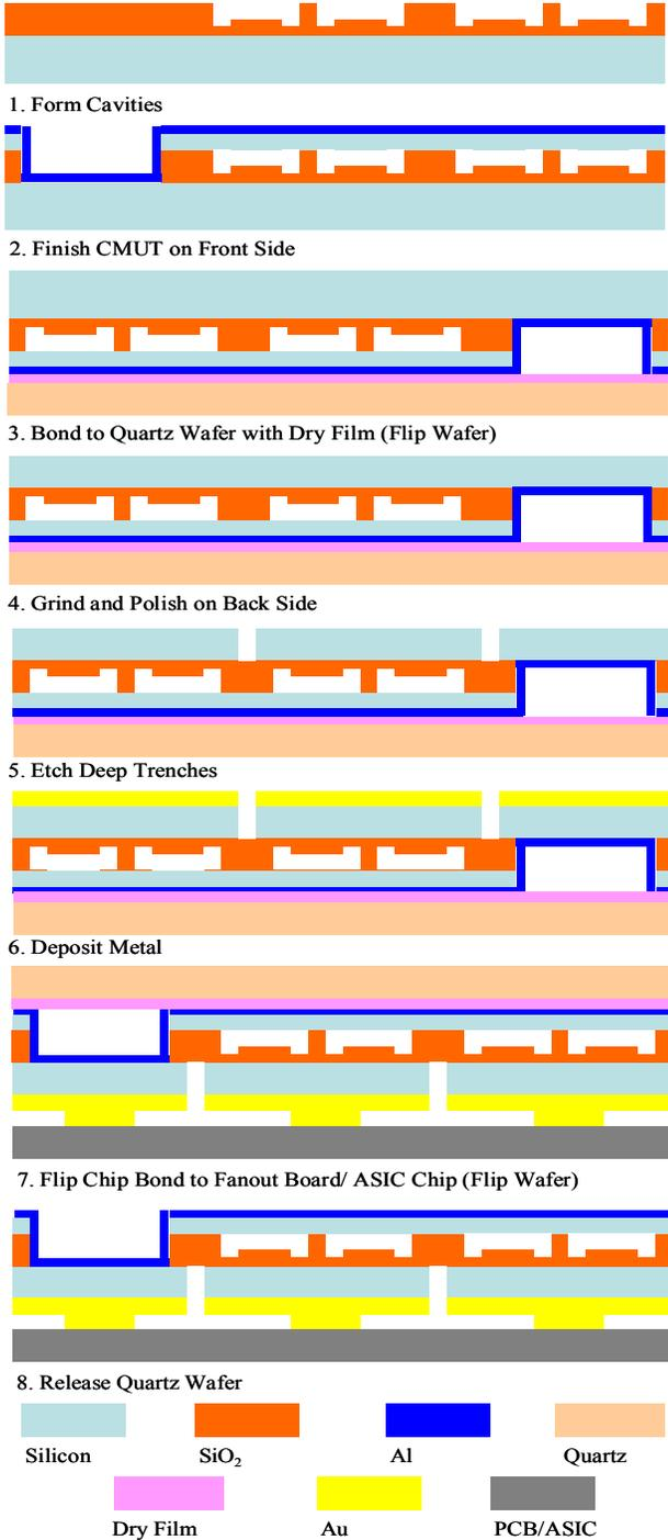
Figure 1: Fabrication steps for through-wafer trench-isolated CMUT arrays.
