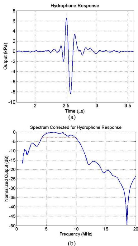
Figure 7: (a) Hydrophone measurement; (b) corresponding spectrum.
