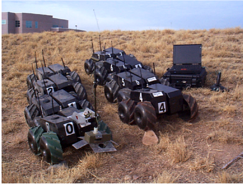
Figure 8: Robotic vehicles in concert can move larger objects, guard a perimeter, perform surveillance, find land mines, or localize a plume of gas, liquid, or radio waves. [138]
