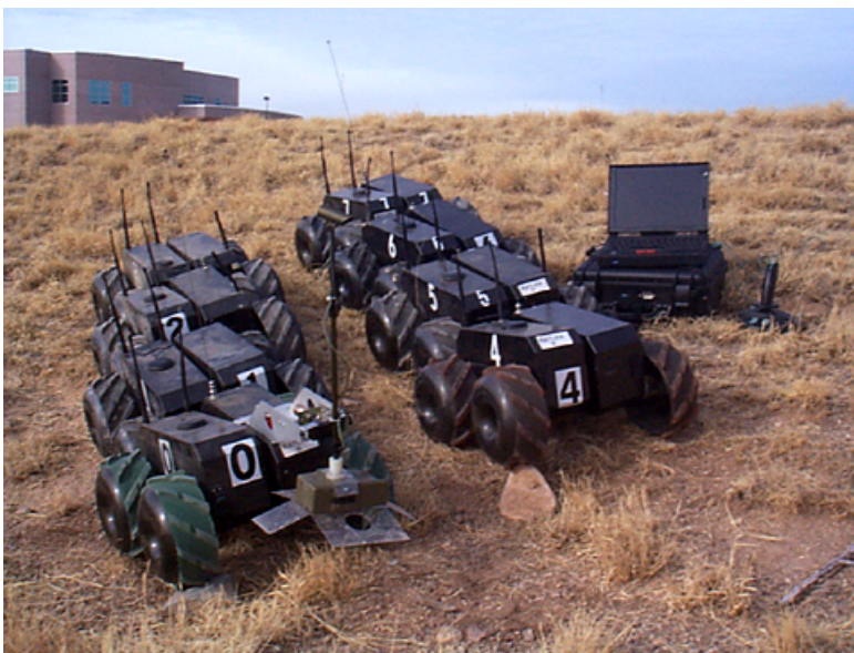
Figure 8: Robotic vehicles in concert can move larger objects, guard a perimeter, perform surveillance, find land mines, or localize a plume of gas, liquid, or radio waves. [121]
