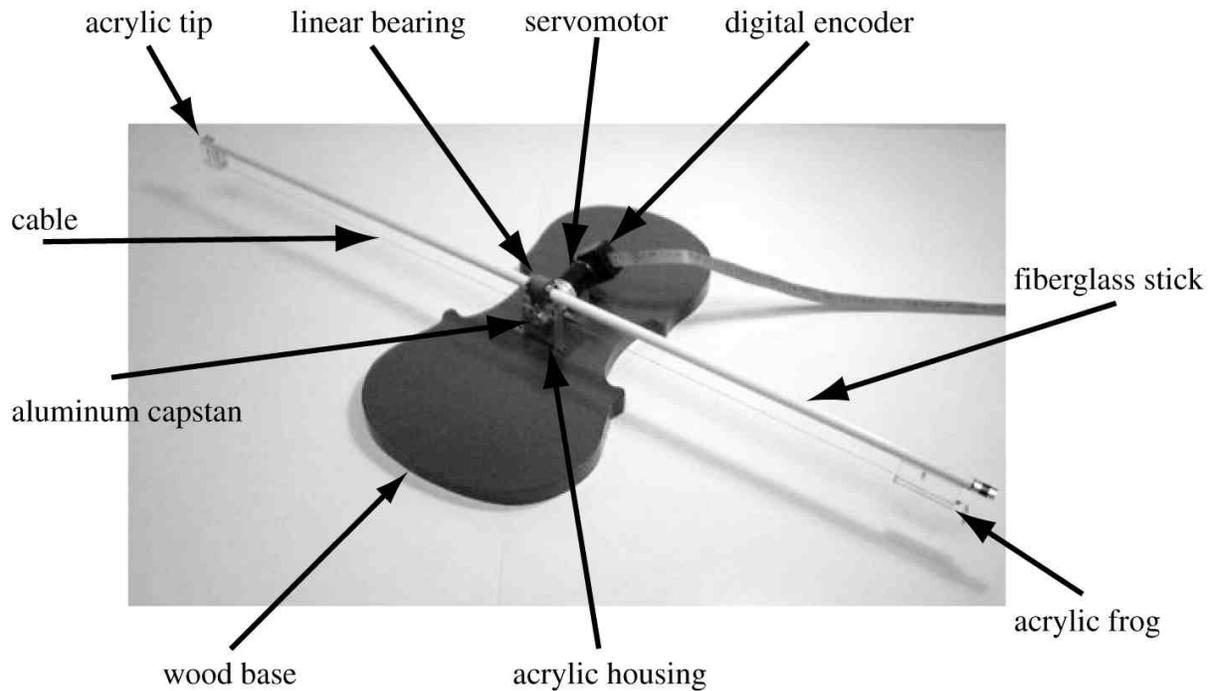
The electronics for the vBow system are comprised of a Maxon Precision Motors linear servo amplifier, single output power supply, and a Servo To Go servo control and data acquisition card installed in a personal computer running the Windows 98 operating system. The servo amplifier, powered by the power supply, amplifies the control signal from the Servo To Go card, for the servomotor. The power for and data from the digital encoder, are provided and decoded by the Servo To Go card.
