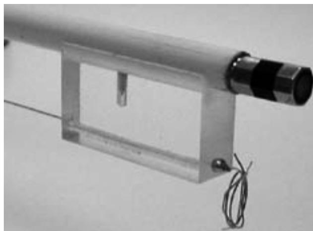
**Figure 4:** The frog with cable tensioner.
