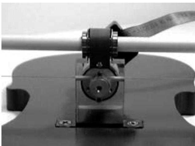
**Figure 2:** The housing for the linear bearing and servo, with holes for the capstan and cable.
