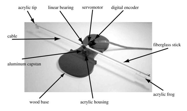
The electronics for the vBow system are comprised of a Maxon Precision Motors linear servo amplifier, single output power supply, and a Servo To Go servo control and data acquisition card installed in a personal computer running the Windows 98 operating system. The servo amplifier, powered by the power supply, amplifies the control signal from the Servo To Go card, for the servomotor. The power for and data from the digital encoder, are provided and decoded by the Servo To Go card.
