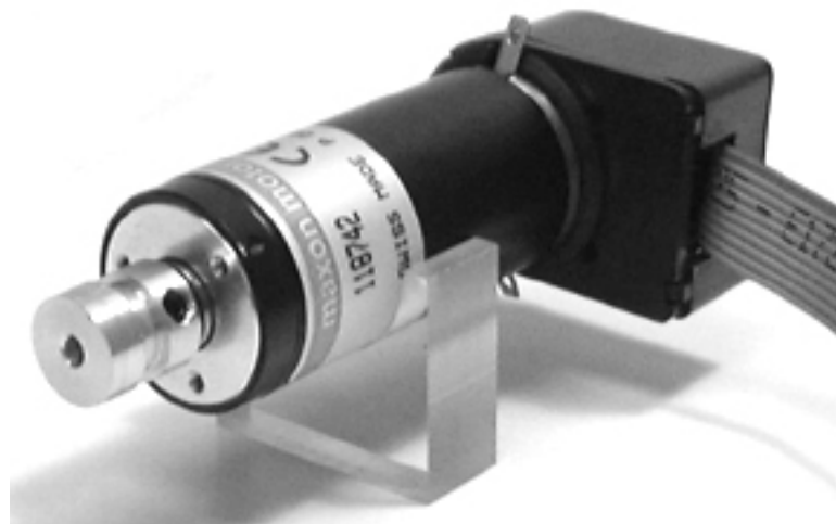
Figure 14. Servomotor with encoder and capstan
