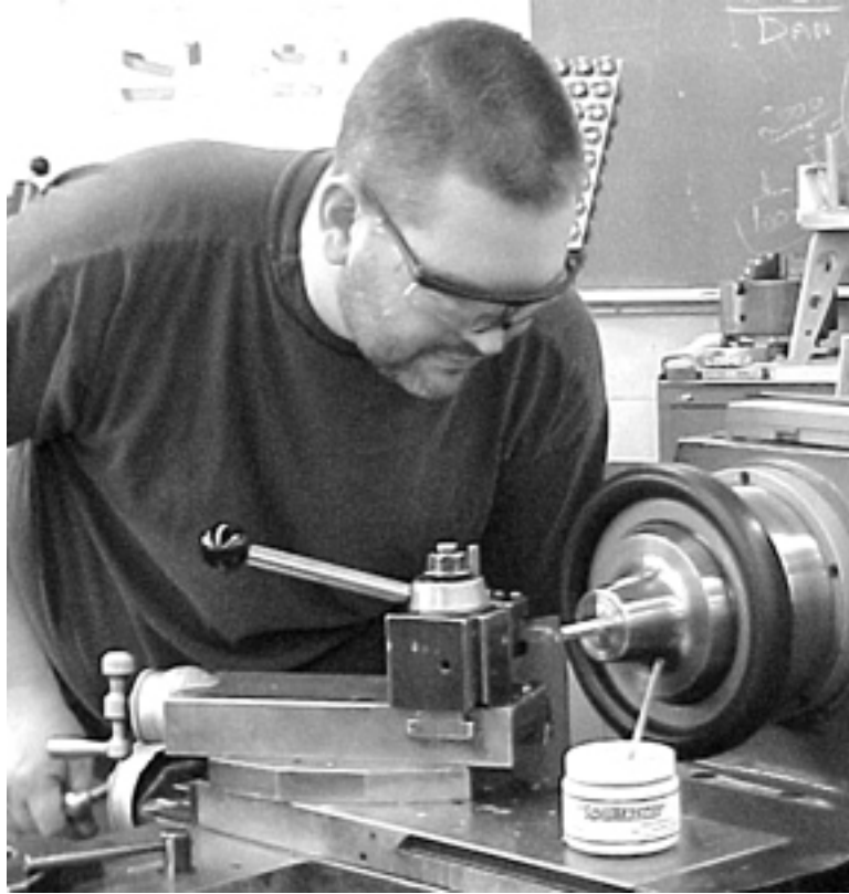
Figure 31. Turning aluminum capstans on a lathe
