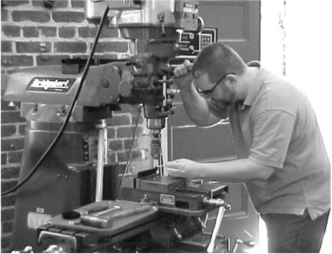
Figure 29. Machining acrylic pieces on a mill
