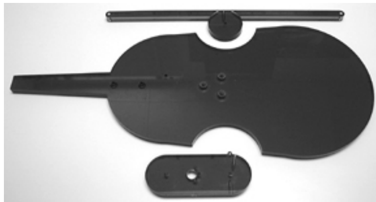
Figure 23: Improved acrylic arm, body, and longitude pieces
