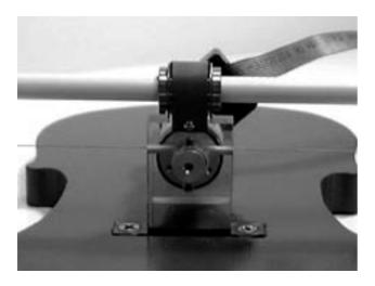
Figure 2: The housing for the linear bearing and servo, with holes for the capstan and cable.
