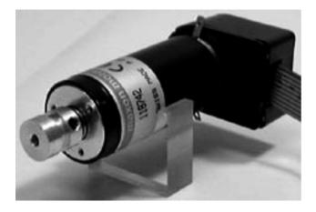
Figure 3: The capstan and servo with encoder.
