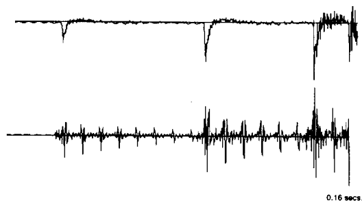
Figure 3: Tone 2. Amplitude plots are shown of first episode (see text) of a note onset at 110 Hz. Top: bridge transducer. Bottom: left-hand index finger accelerometer.
