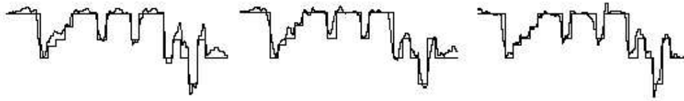
Figure 3. Three theremin performances of the same melody by different subjects under different force conditions (1, 3 and 4, above). Measured pitch curves are shown inscribed over a template computer performance (consisting of instantaneous pitch changes between perfectly tuned pitches).
