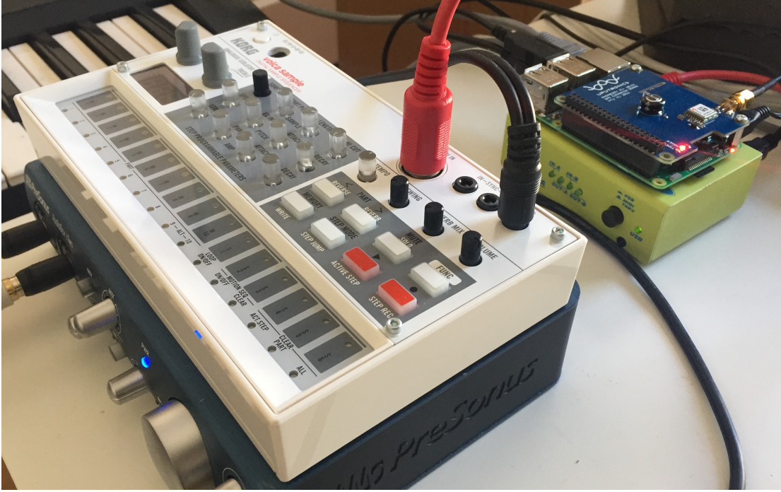
Figure 4.1: An example of a PIGMI set up for working with a MIDI sequenced instrument. Attached to the Raspberry Pi is a Midiman MIDI interface which is connected to a Korg Volca Sample sampling drum machine.
