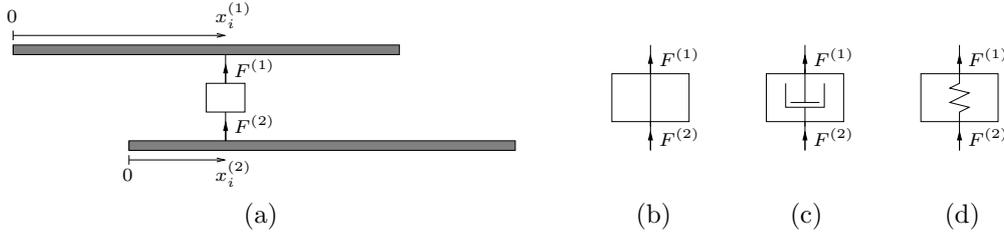
Figure 7.14: (a) A pair of bars, pointwise coupled by an arbitrary mechanism relating the resulting forces. (b) A rigid connection, (c) a damped connection, and (d) a spring-like connection.
