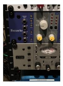
Channels 17-20 can go direct to the DM2000 from the Switchcraft XLR Patchbays
