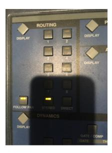
and check that **Stereo** is also selected in the **Control Room** section.
