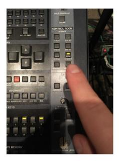
Raise the Stereo Fader and then raise the Control Room Level pot.
