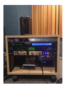
The settings of the MOTU 112D never need to be changed either on the unit itself or on your profile. This MOTU controls the audio in and out for this routing. The MOTU Midi Time Piece will handle Midi in and out to the Live Room/Disklavier.
