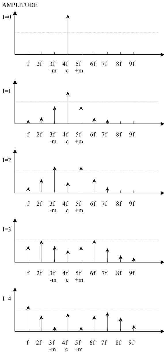
Fig. 5. Plot of spectrum where the ratio of  $c/m$  is  $4/1$ . As the index increases, the reflected lower side frequencies begin to affect the spectrum when  $I = 3$ , where the fundamental,  $c-3m$ , is noticeably greater than the 7th harmonic,  $c+3m$ .
