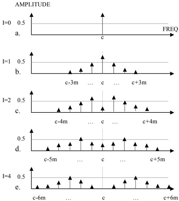
Fig. 1. Example to show increasing bandwidth with increasing modulation index,  $I$ . The upper and lower side frequencies are at intervals of the modulating frequency,  $m$ , and are symmetrical around the carrier,  $c$ .
