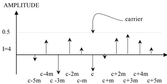
Fig. 3. Plot of Fig. 1e with phase information included (modulation index = 4). The bars extending downward represent spectral components whose phases differ by 180°.
