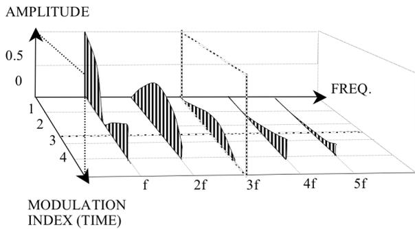
Fig. 7. Dynamic spectrum where the ratio  $c/m = 1/1$  and the modulation index increases from 0 to 4 continuously. The increasing bandwidth of the spectrum is clearly seen, but because of the reflected side band frequencies, the evolution of the individual components is not intuitively clear.
