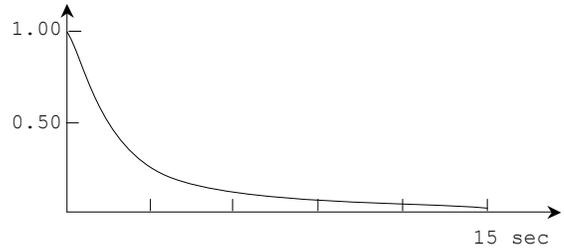
Fig. 14. Exponentially decaying envelope for bell-like timbres
