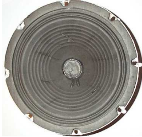
Figure 13: Mishandled driver with additional cuts in the cone
