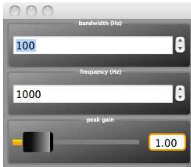
Figure 12: Main (and only) window of a Qt application generated by faust2jaqt from cpgrui.dsp on a Mac OS X system.
