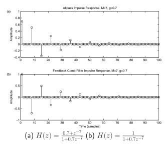
• Steady-state tones (sinusoids) really do see the same gain at every frequency in an allpass, while a comb filter has widely varying gains.
