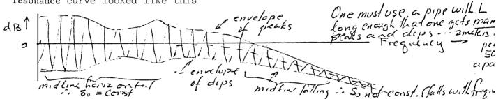
Do not forget that even if the capillary is not frequency-independent, , its behavior is smooth enough that a simple RC equalizing circuit can usually be designed for use in either the excitation feedback loop or in the pressure microphone channel to get an effectively constant system.
