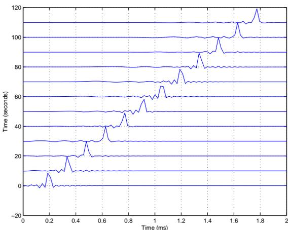
**Fig. 1:** Recorded Impulse Train with Clock Drift. A two-minute long recorded impulse train in the presence of clock drift.
