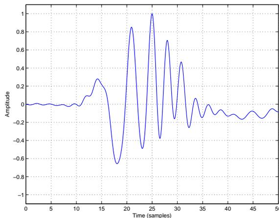
**Fig. 6:** Impulse Response Direct Path With Clock Drift. The direct path of an impulse response in the presence of clock drift used for comparison with Fig. 7 and Fig. 8.
