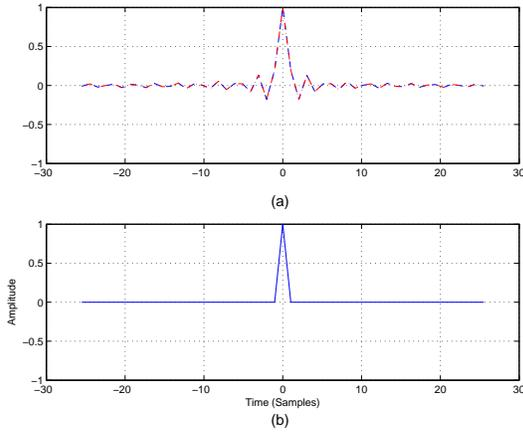
**Fig. 3:** (a) Impulse Responses Using Time-Reversal Mirror and Closed-Form Inverse Approaches. Impulse responses computed using inverse filters via time-reversal mirror (dashed dot) and closed-form inversion (dashed) approaches showing roughly bandlimited inversion. (b) Impulse Response Using the Numerical Inversion Inverse Approach. An impulse response computed using an inverse filter created via numerical inversion showing an improved result.
