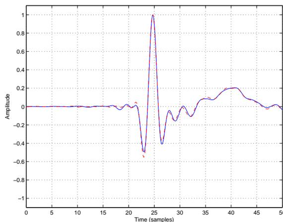
**Fig. 7:** Impulse Response with Compensation. Impulse response with drift compensation (dashed) using explicit clock drift estimation and windowed sinc interpolation plotted against a reference impulse response with no drift (solid).
