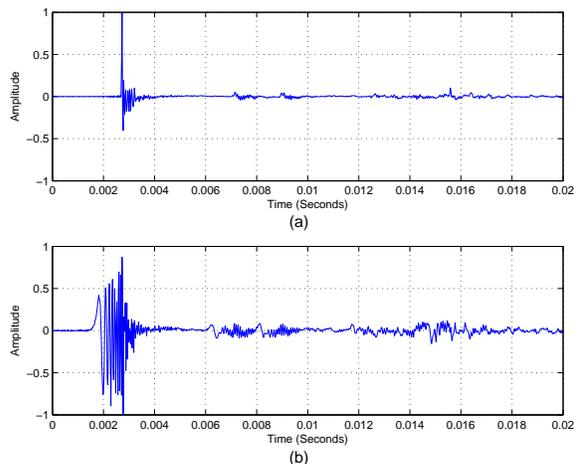
**Fig. 2:** (a) Room Impulse Response without Clock Drift. A reference room impulse response measured without clock drift using a single audio interface for playback and recording. (b) Room Impulse Response with Clock Drift. A room impulse response measured in the presence of clock drift using two unsynchronized audio interfaces for playback and recording.
